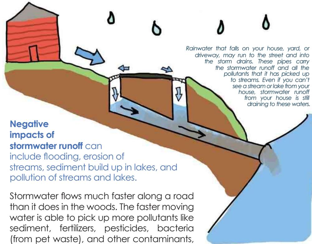
Rainwater that falls on your house, yard, or driveway, may run to the street and into the storm drains. These pipes carry the stormwater runoff and all the pollutants that it has picked up to streams. Even if you can't see a stream or lake from your house, stormwater runoff from your house is still draining to these waters.
